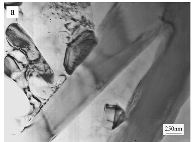
Fig. 8. Back-scattered electron morphology of interfacial reaction layer.
